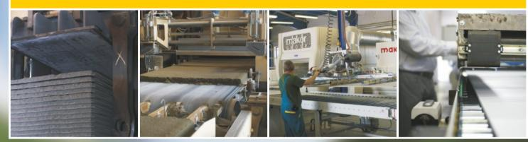
**CETRIS®** cement bonded particleboards are produced by pressing a mixture of wooden particles and portland cement with water. The surface is smooth, the color is cement-like grey.
